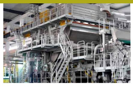
energy efficiency, as stated, is to dry with the Yankee alone with the hood just providing suction, but to respect a mill's needs both for energy efficiency and output, a hybrid solution can be ideal.
