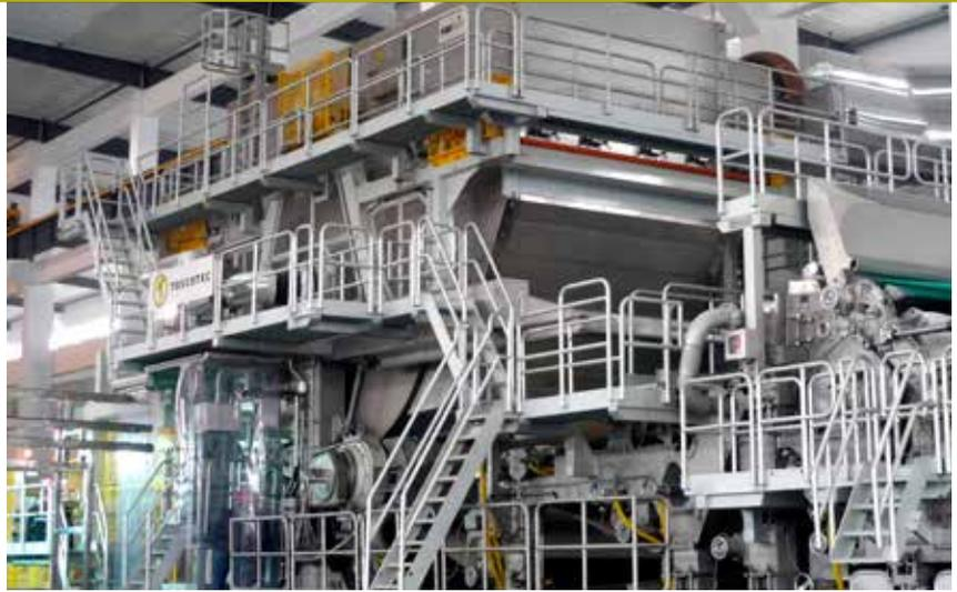
energy efficiency, as stated, is to dry with the Yankee alone with the hood just providing suction, but to respect a mill's needs both for energy efficiency and output, a hybrid solution can be ideal.
