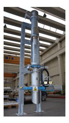
Additionally, the heavy rejects trap is provided with sight glasses. These features, together with the rotor-less concept, make the TT HighDensityCleaner very easy to operate and quick to maintain. Moreover the fiber losses are minimized thanks to the reject trap design.
