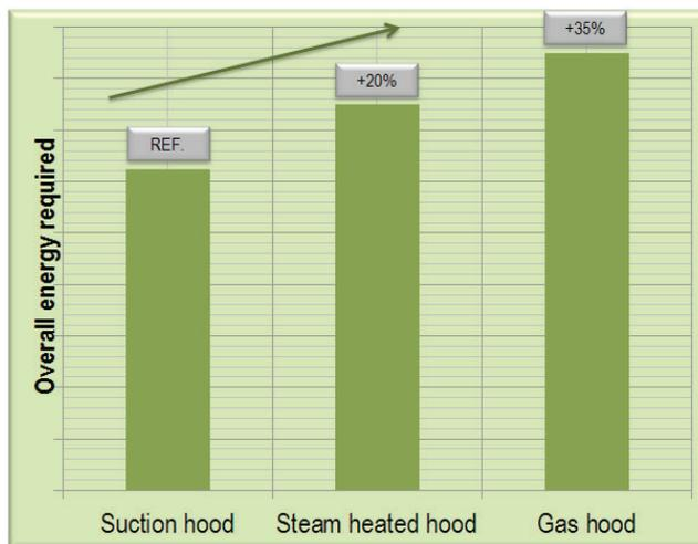
heat-resistant insulation panels, accompanied by stable containment of this insulation material, are essential factors to guarantee the maximum effectiveness of the hood insulation. Given the optimum Steel Yankee Dryer, it is the hood which completes the picture in the drying section. Choice of hood is not straightforward, because there are many options.
