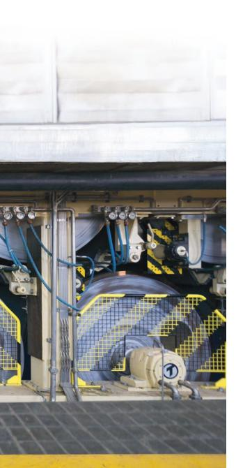
surface than cast iron dryers of the same face length. Basically, maintaining unchanged the overall length of the dryer section of the paper machine, we significantly increased our drying capacity, due to the larger diameter and drying surface of the new steel dryers. As a result, we were also able to preserve our existing hood, which is still working well. Toscotec had many successful references of similar rebuild projects and we were rather impressed with their extensive experience.
