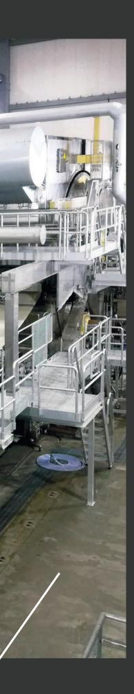
its load and tilt, TT NextPress delivers highly consistent moisture across the sheet and a softer and bulkier tissue, while ensuring maximum energy efficiency in the drying process.
