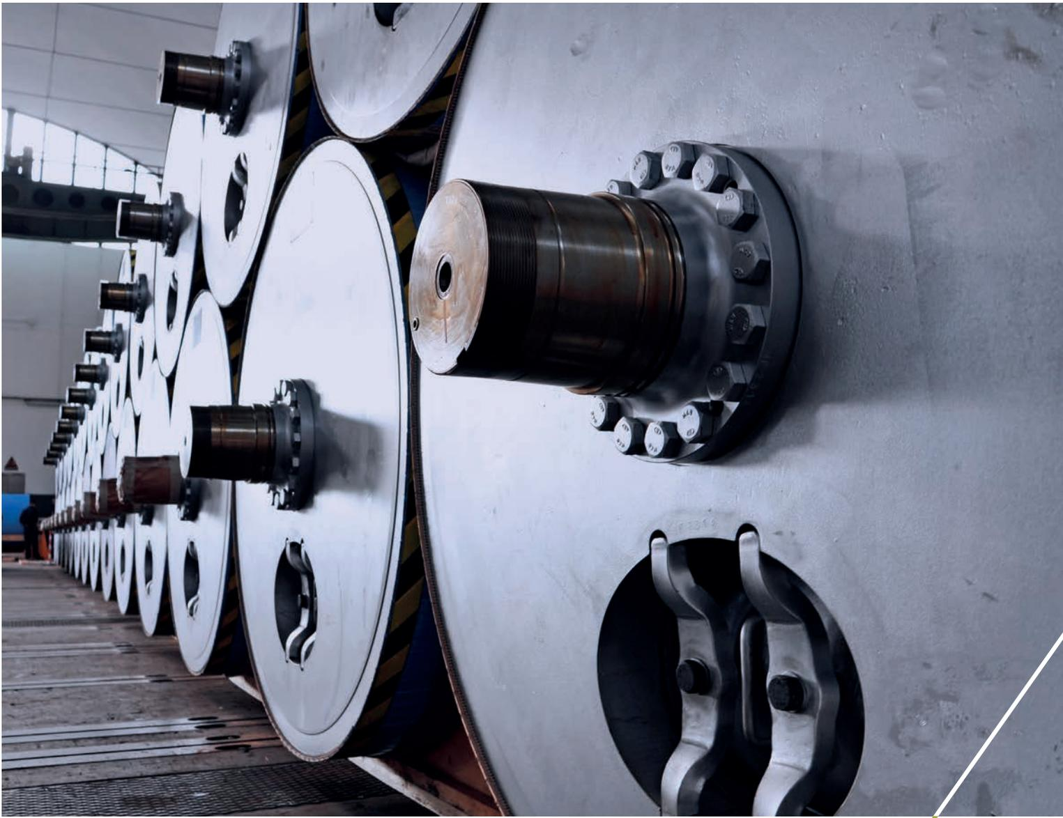
the rebuilding is to implement machine efficiency, reliability and safety in operations. Toscotec's delivery includes 25 new TT SteelDryers in place of casted iron dryers, that will allow the paper mill to increase its drying capacity, production and the width of the paper produced. The existing mechanical drive will be replaced with a new silent drive system. Tail threading will be ropeless from the press section through the new dryer section up to the pope reel.
