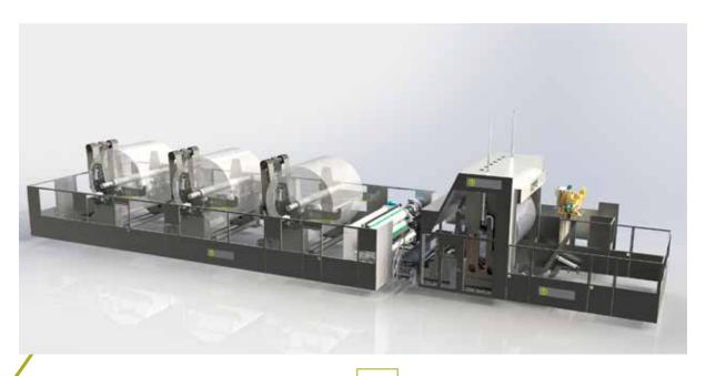
On July 27, Hygienic Tissue Mills started up a Toscotec-supplied TT WIND-P tissue rewinder at its Pietermaritzburg mill, in eastern South Africa. This is a repeated order for Toscotec, following the supply of a MODULO-PLUS tissue machine, PM2, in 2017. The TT WIND-P slitter rewinder serves PM2, processing 100% virgin pulp and recycled paper parent rolls.
