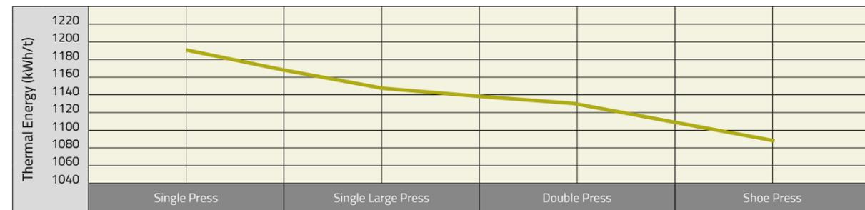
The diagram above is based on a standard Steam Hood configuration and a 5.5m (18FT) Steel Yankee. The post press dryness has a direct impact on the overall energy required in thermal drying. The use of a large diameter press can lead to reduced water content in paper entering the Yankee. 1% dryness increase can result in overall energy reduction of 4% to 7%.
