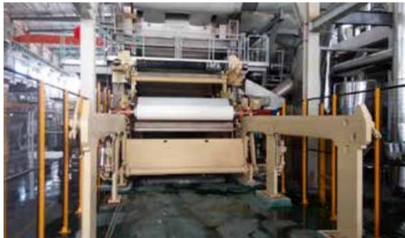
increase the company's tissue production by 42,000 t/y. Toscotec's scope of supply includes a MODULO-PLUS ES machine, designed for a speed of 1500 m/min, featuring TT SYD-15FT (4572mm) and double press configuration, Milltech's steam-heated hood, stock preparation equipment, electrical and control systems, spare parts for the entire plant and a full service package.
